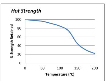
"Hot strength" shear strength tests performed on mild steel. Fully cured then conditioned to pull temperature for 30 minutes before testing. ES566 can withstand higher temperatures for brief periods (such as for paint baking and wave soldering processes) providing the joint is not unduly stressed. The minimum temperature the cured adhesive can be exposed to is -40°C (-40°F) depending on the materials being bonded.
