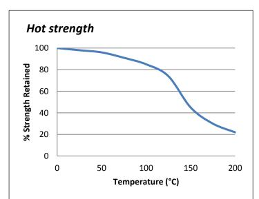
"Hot strength" shear strength tests performed on mild steel. Fully cured then conditioned to pull temperature for 30 minutes before testing. ES560 can withstand higher temperatures for brief periods (such as for paint baking and wave soldering processes) providing the joint is not unduly stressed. The minimum temperature the cured adhesive can be exposed to is -40°C (-40°F) depending on the materials being bonded.
