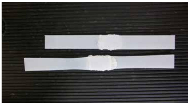
Polypropylene lapshears bonded with TA4610 - the adhesive bond is so strong the plastic stretches and deforms and suffers failure before the joint.
