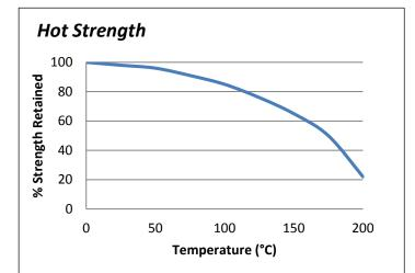
"Hot strength" shear strength tests performed on mild steel. Fully cured then conditioned to pull temperature for 30 minutes before testing. ES5691 can withstand higher temperatures for brief periods (such as for paint baking and wave soldering processes) providing the joint is not unduly stressed. The minimum temperature the cured adhesive can be exposed to is -40°C (-40°F) depending on the materials being bonded.
